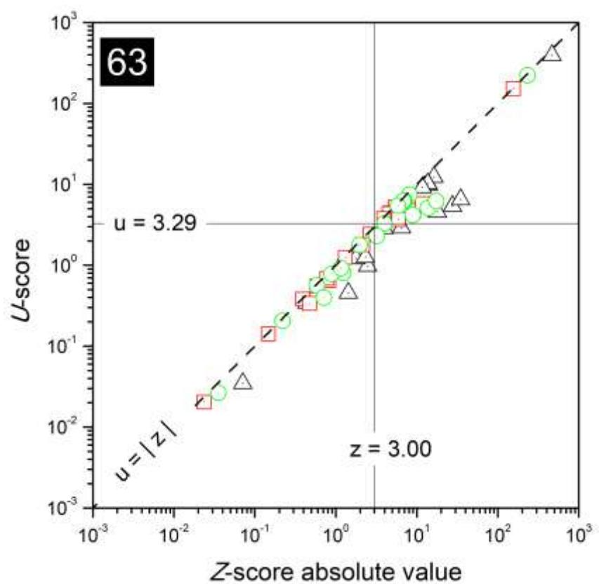
FIG. 66. Combined plots of  $z$ - and  $u$ -scores for the laboratory with code 63.
