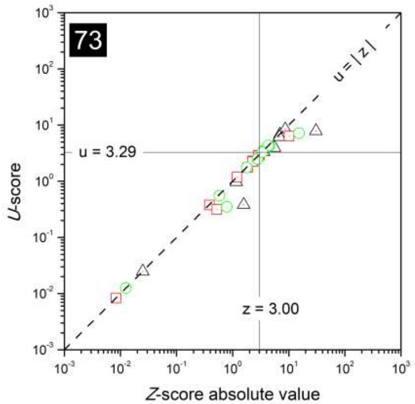
FIG. 71. Combined plots of  $z$ - and  $u$ -scores for the laboratory with code 73.
