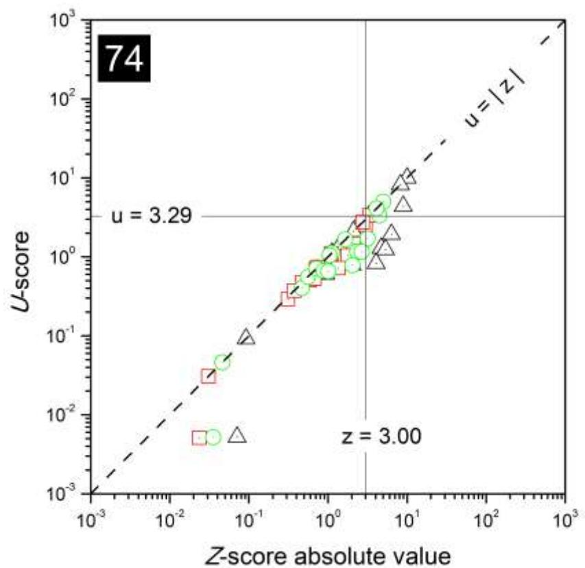
FIG. 72. Combined plots of  $z$ - and  $u$ -scores for the laboratory with code 74.
