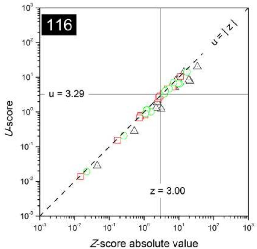
FIG. 91. Combined plots of  $z$ - and  $u$ -scores for the laboratory with code 116.
