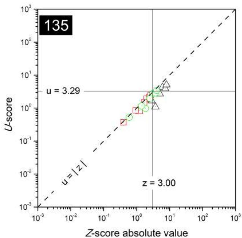
FIG. 104. Combined plots of  $z$ - and  $u$ -scores for the laboratory with code 135.
